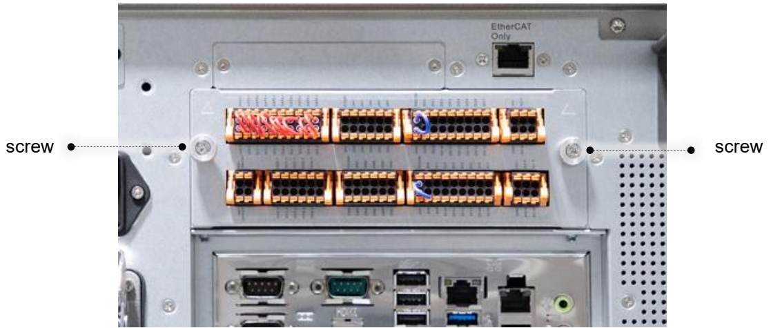
Figure 55: Detachable I/O Panel
