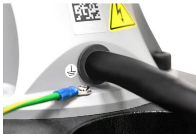
Figure 13: Securing the ground wire with the robot
